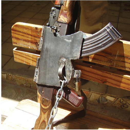
Safe gun clamp designed by DDG for use by communities in Somaliland. Photo courtesy of DDG-Somaliland
